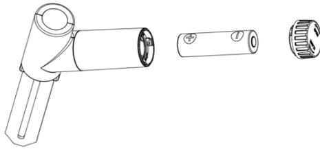
1. Open the battery cap of the soil moisture sensor
